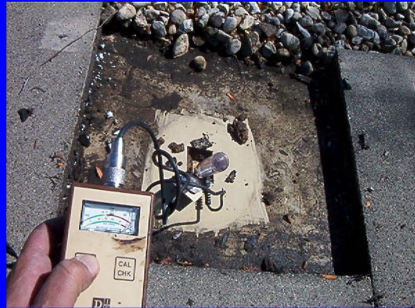
Moisture Meters are used to verify if there is wet insulation at locations indicated by the infrared scan. Cores are taken to determine the type of insulation and the amounts of roofing on the building as well as the deck type and attachments.
